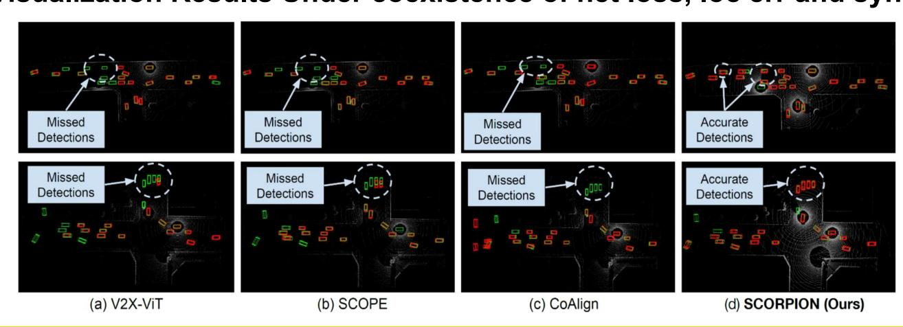
SCORPION outperforms baselines under various levels of network loss & loc/sync errors
