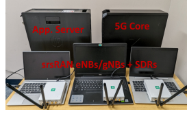
Fig. 9. The over-the-air prototype testbed of OPCM.
